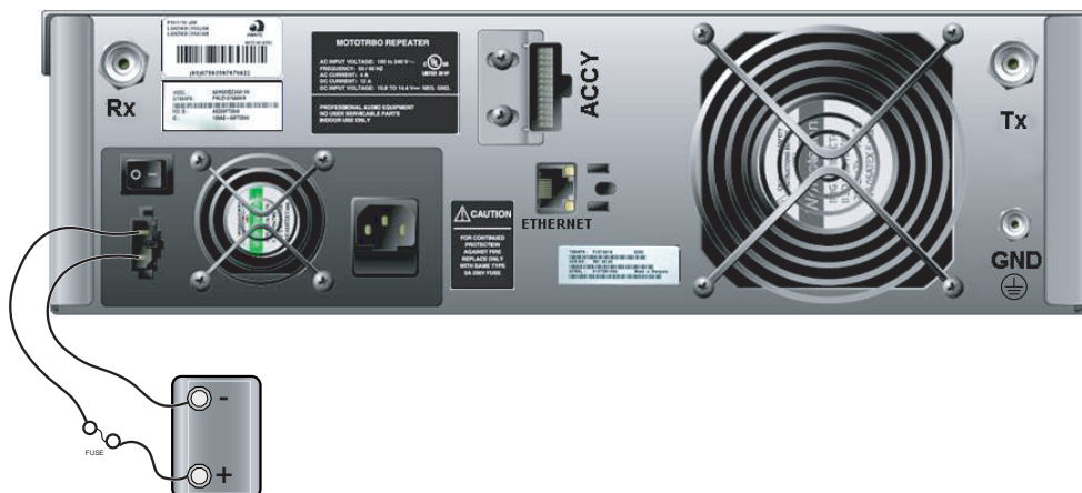
Figure 4-2 Making Connections to a Backup Battery
